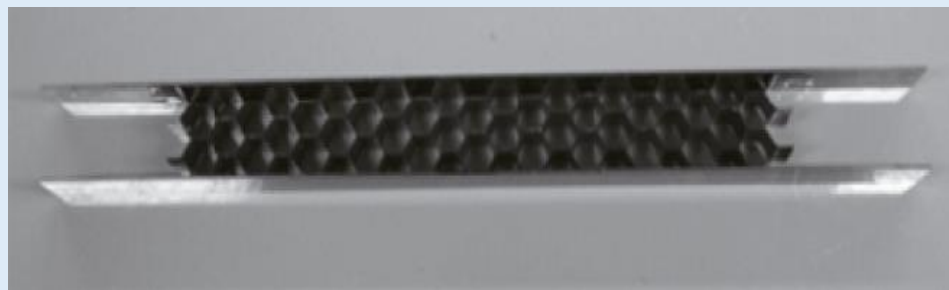
SMA honeycomb core actuator [Okabe, 2011]
