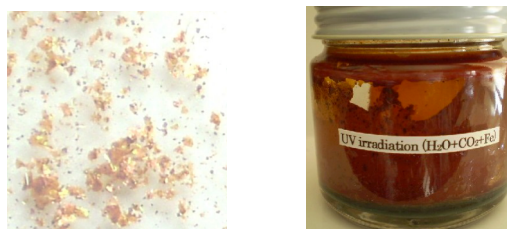
Fig. 4 (a) Dried floating materials. (b) Membrane on a wall. Fig.4 (a) is the photo on the dried floating materials made from carbonated water and steel wool. Fig.4 (b) is the photo on the membrane that was formed by adhering to the wall of the glass in 90 cc of carbonated water mixed with 5 g of #300 iron powders.
