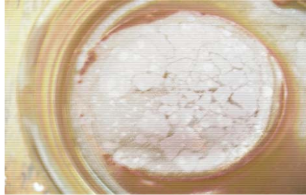
Fig. 5. The membrane that is obtained by irradiation of ultraviolet rays. The membrane is easy to break.
