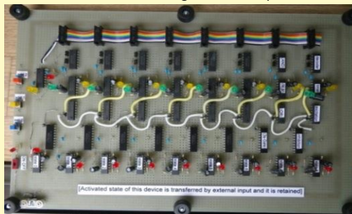
Fig.4 A state transition circuit that is made of mono multi vibrators.
