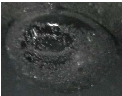
Fig. 33 The substance that adhered to a glass wall (the photographing is after 10 hours 27 minutes from the mixing, iron powder and CaCO 3 were mixed with carbonated water)
