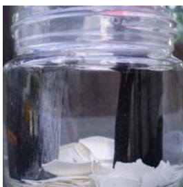
Fig.20 An electrode changes by electric current in the carbonated water with calcium carbonate.
