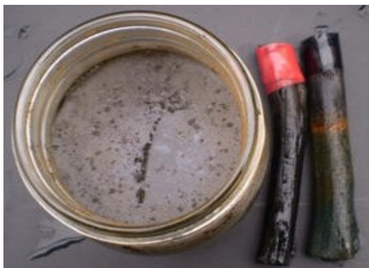
Fig.19 The products of electrolysis processing of water solved with iron by using carbon electrodes are similar to the products in carbonated water mixed with iron powder.
