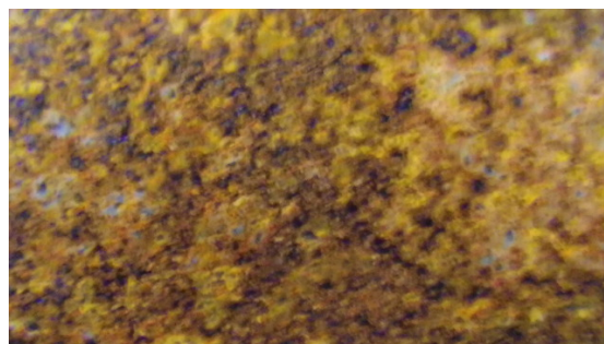
(a) Fe mixed with \text{CO}_2 in a glass container (b) iron oxide on the glass wall
