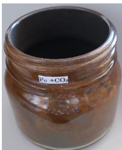
(a) Fe mixed with \text{CO}_2 in a glass container (b) iron oxide on the glass wall
