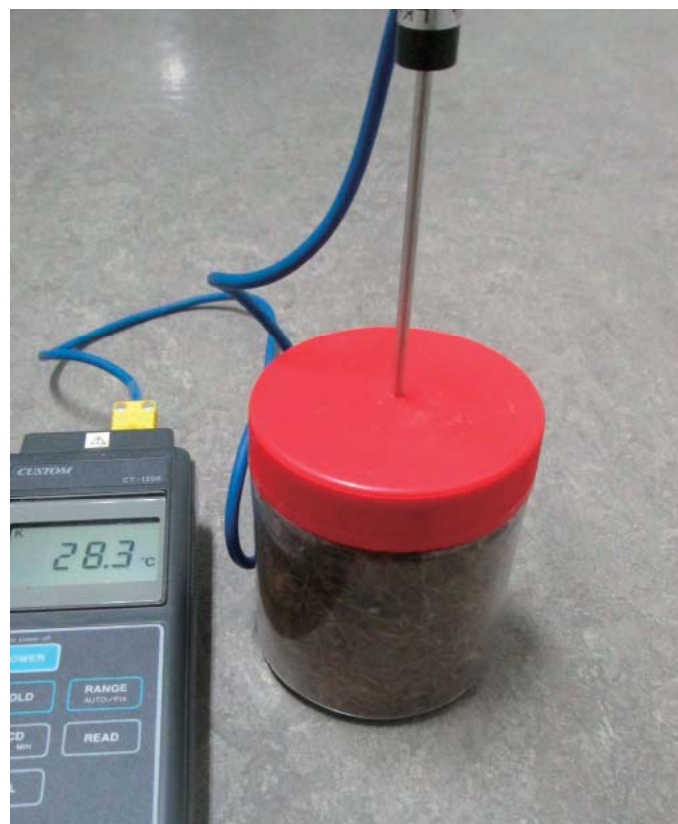
Fig.1 Method of measuring temperature of bark fibers in the vessel. Temperature sensor is inserted through the vessel cap hole to the center of bark fibers in the vessel.
