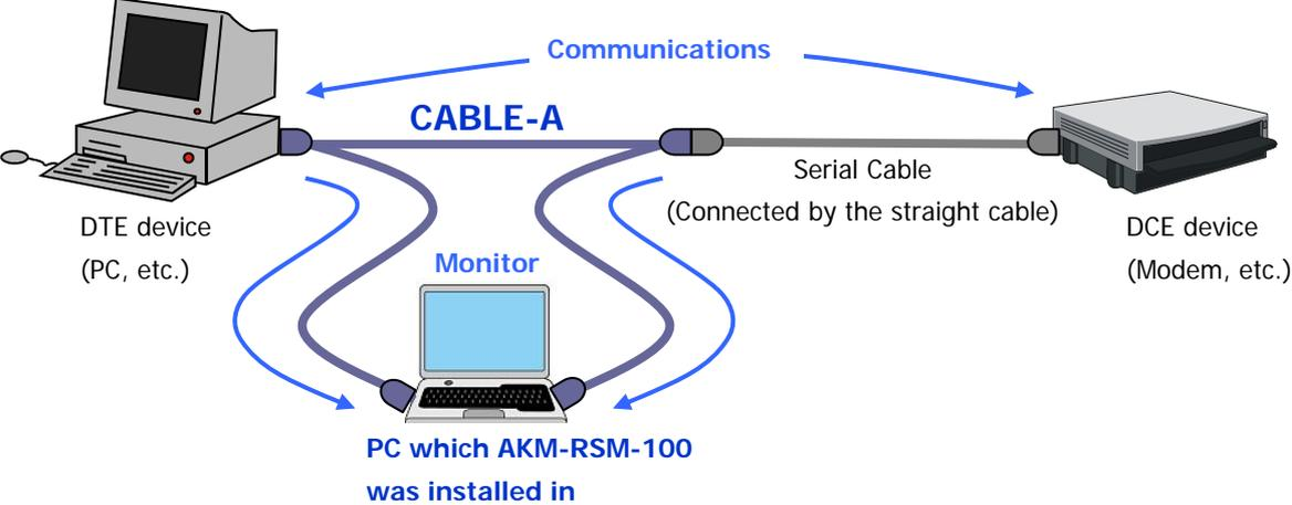
■ Direct Connection (DTE-DCE connection) \*Note: CABLE-A is used.
