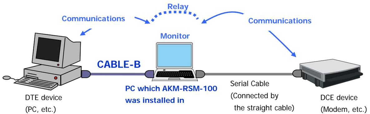
■ Relay Connection (DTE-DTE connection) \*Note: CABLE-B is used.
