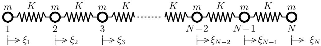
$$\begin{aligned} m \frac{d^2}{dt^2} \xi_1 &= -K(\xi_1 - \xi_2) \\ &\dots \\ m \frac{d^2}{dt^2} \xi_r &= -K(-\xi_{r-1} + 2\xi_r - \xi_{r+1}) \\ &\dots \\ m \frac{d^2}{dt^2} \xi_N &= -K(-\xi_{N-1} + \xi_N) \end{aligned} \quad (33)$$
