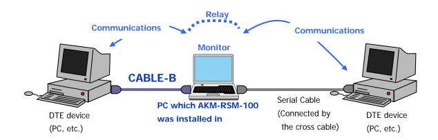
(Note) The "Relay Connection" is used for the Support of Debugging to do the increase in efficiency of software development and to do the support of the trouble solution of the DTE device side and the DCE device side, too.
