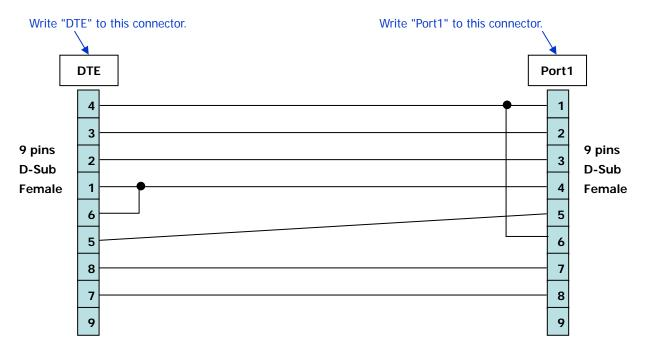
(Note) Be careful of the pin numbering on the DTE side.
